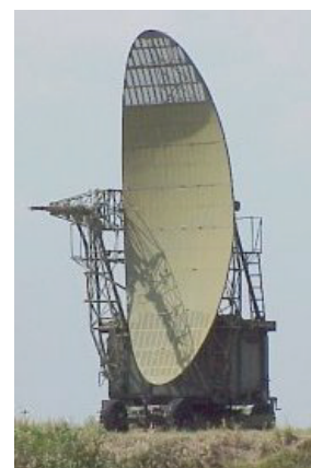
Russian height-finding Radar with nodding antenna “Odd Group”
